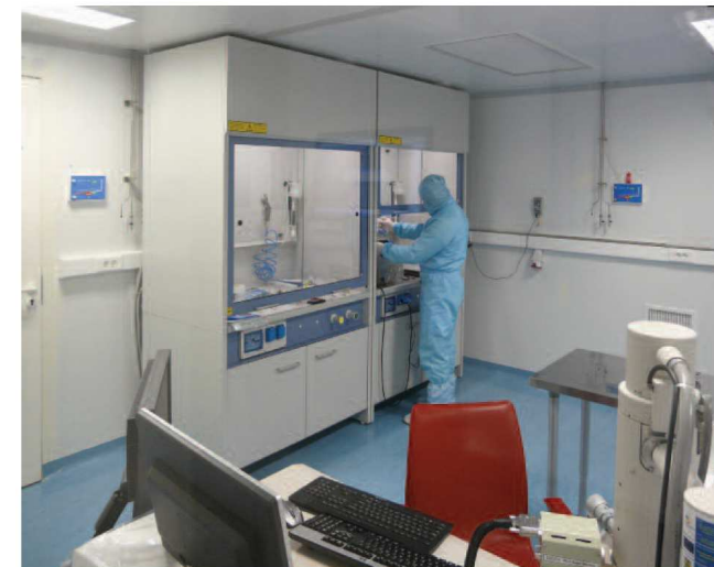
The new clean room facility including: photolithography (EVG620); nanolithography (Hitachi S3400N+Raith Elphy Quantum); metallization plants (BESTEC).
