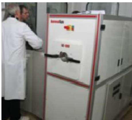
Equipment for low pressure chemical vapor deposition of thin layers LPCVD, AnnealSYS
