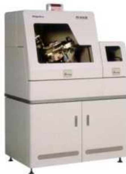
THz-TDS instrument from Aispec (from 40 GHz up to 7 THz)
